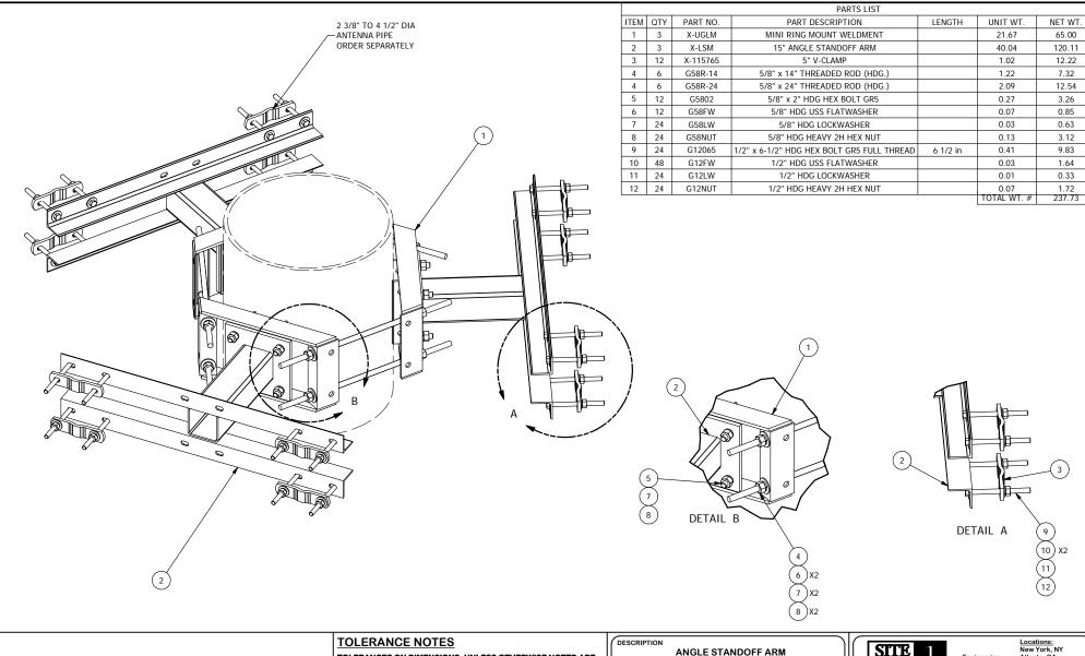
TOLERANCES ON DIMENSIONS, UNLESS OTHERWISE NOTED ARE: SAWED, SHEARED AND GAS CUT EDGES (± 0.030") DRILLED AND GAS CUT HOLES (± 0.030") - NO CONING OF HOLES LASER CUT EDGES AND HOLES (± 0.010") - NO CONING OF HOLES BENDS ARE ± 1/2 DEGREE
